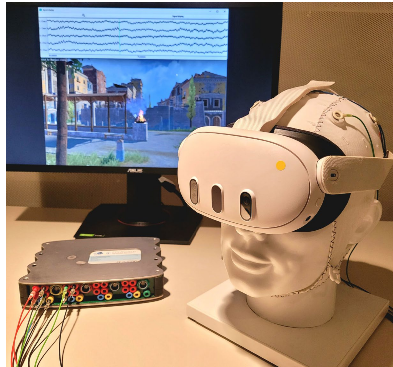
Figure 1. Schematic setup of a combined VR-EEG measurement, where the VR scenario displayed within the VR headset and the recorded EEG traces are simultaneously shown on a screen in the background.
